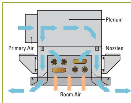
**Figure 30:** Air flow diagram of a typical linear active beam in cooling
