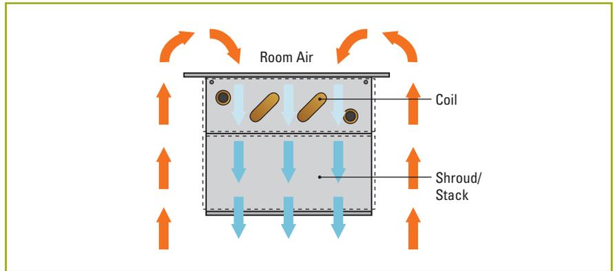
**Figure 20:** Passive beam air flow pattern
