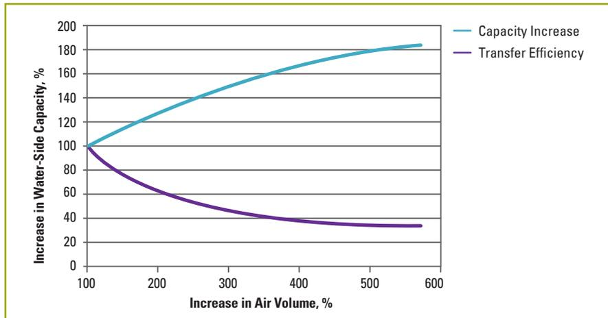
**Figure 34:** Capacity vs. air volume
