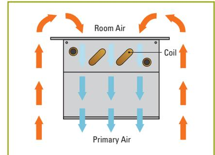
**Figure 2:** Air flow diagram of a passive chilled beam in cooling
