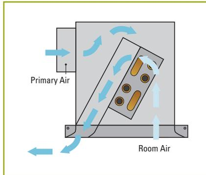
**Figure 13:** Air flow diagram of a linear active beam in cooling with 1 way discharge
