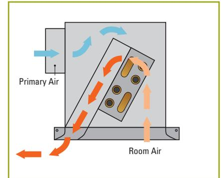
**Figure 14:** Air flow diagram of a linear active beam in heating with 1 way discharge
