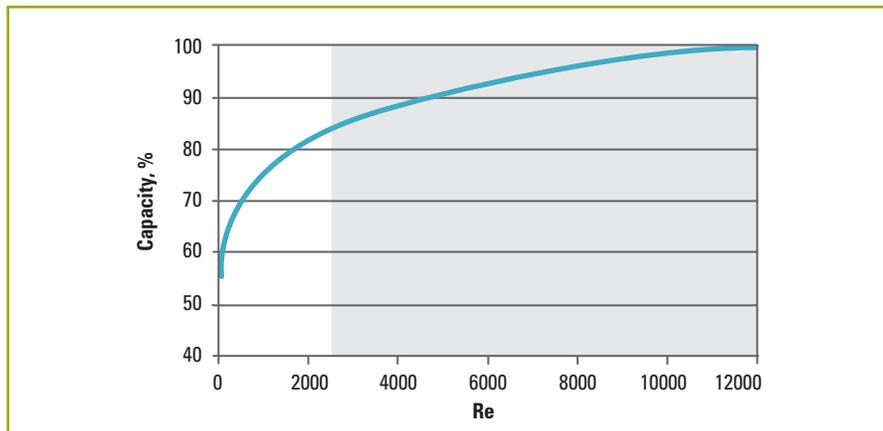
**Figure 18:** Passive beam capacity vs. water flow
