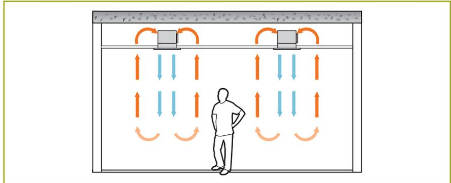
**Figure 5:** Room air flow pattern of a passive beam in cooling
