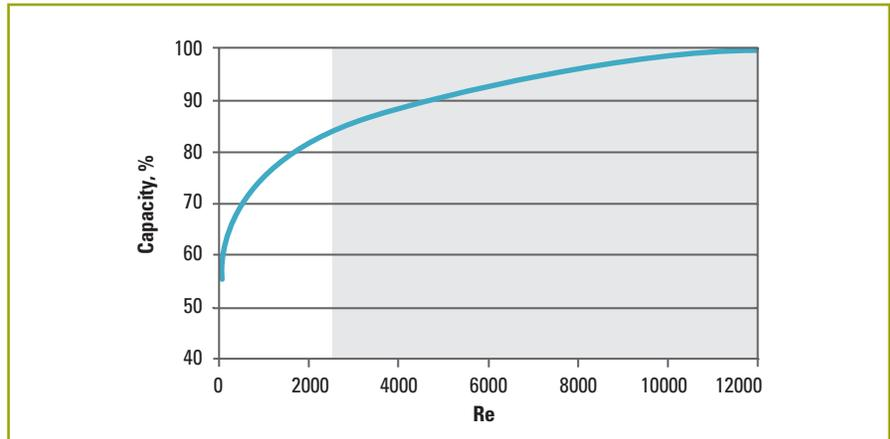
**Figure 35:** Active beam capacity vs. water flow
