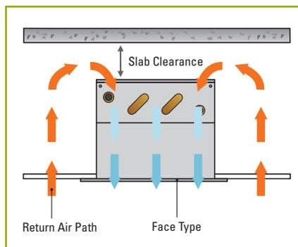
**Figure 22:** Factors that affect performance of passive beams
