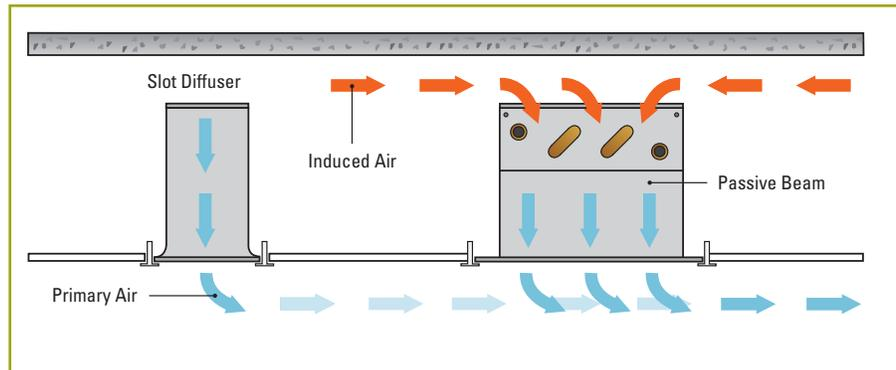
**Figure 25:** Inducing air through the passive beam with increased velocity across the face
