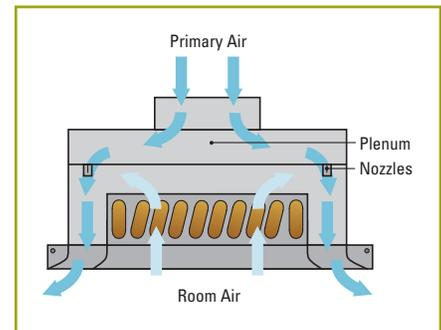
**Figure 31:** Air flow diagram of a modular active beam in cooling
