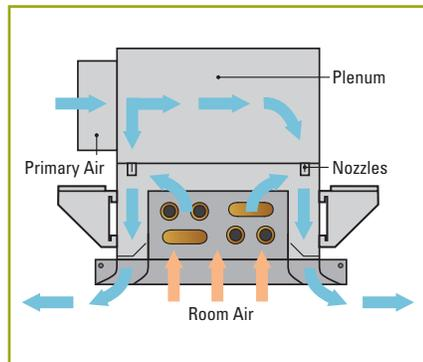
**Figure 10:** Air flow diagram of a typical linear active beam in cooling
