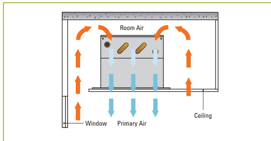
**Figure 26:** Capturing the plume at the perimeter may increase passive beam performance
