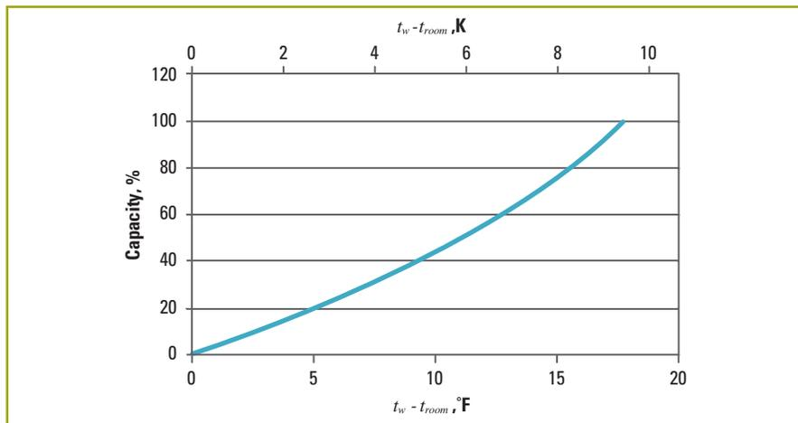
**Figure 19:** Passive beam capacity vs. difference between mean water and room air temperature
