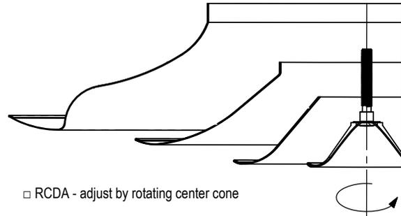
RCDA - adjust by rotating center cone
