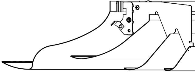
RCD - adjust by repositioning cone mounting brackets
