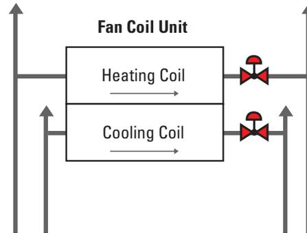
Figure 20: Common Coil 4 Pipe System
