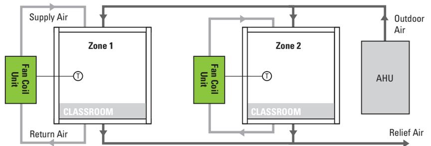
**Figure 3:** Outdoor air ducted into fan coil unit
