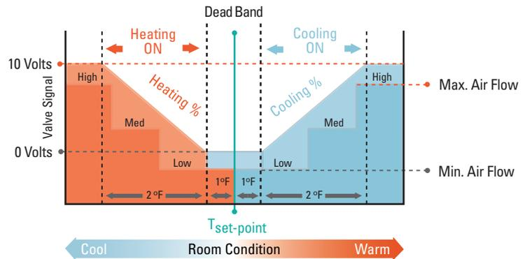
**Figure 29:** Sequence of operation for automatic heat /cool changeover, modulating control of heating and cooling with discharge air temperature control of the cooling and heating flow and variable fan speed.
