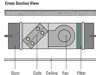
**Figure 6:** Horizontal Concealed Fan Coil
