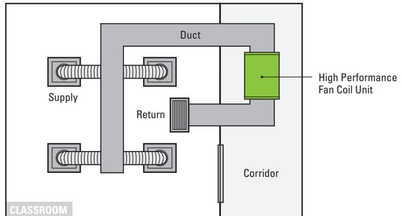
**Figure 9:** Horizontal High Performance Fan Coils
