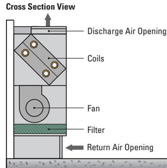
**Figure 5:** Horizontal Fan Coil Arrangement
