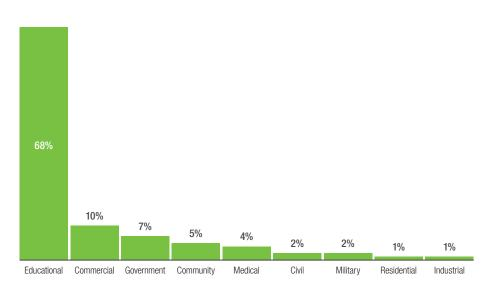
**Table 1:** Building types and percentage of total building types using chilled beams (2012 to 2014\*)
