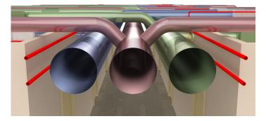
Figure 3: Hospital patient room hall interstitial space for an all-air system (supply duct, exhaust duct, and return duct)
