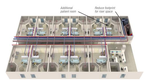
Figure 2: Reduced riser and mechanical room space requirements could allow for an additional patient room on each floor
