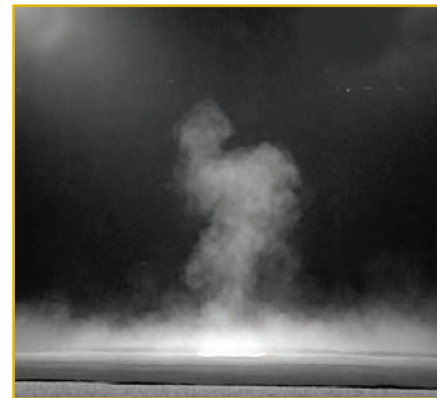
Figure 15: Flow diffuser air pattern
