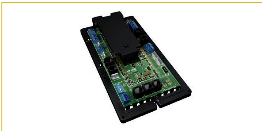
Figure 42: Underfloor terminal unit controller
